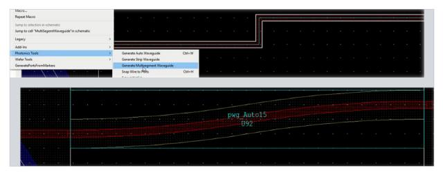
Creating a waveguide in L-Edit Photonics is a two step process. First, create an orthogonal route that connects the two components. Then, by pressing a hot key, that route can be converted into a waveguide with the appropriate curvatures, based on the process.
