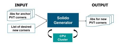
Generator builds a machine learning model of the library to produce production-accurate Liberty models at new PVT corners 100x+ faster than SPICE.
