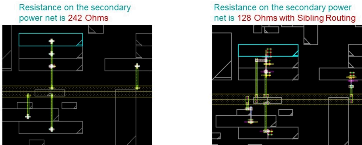
Figure 12. Resistance on secondary power nets with regular routing vs. sibling routing.
